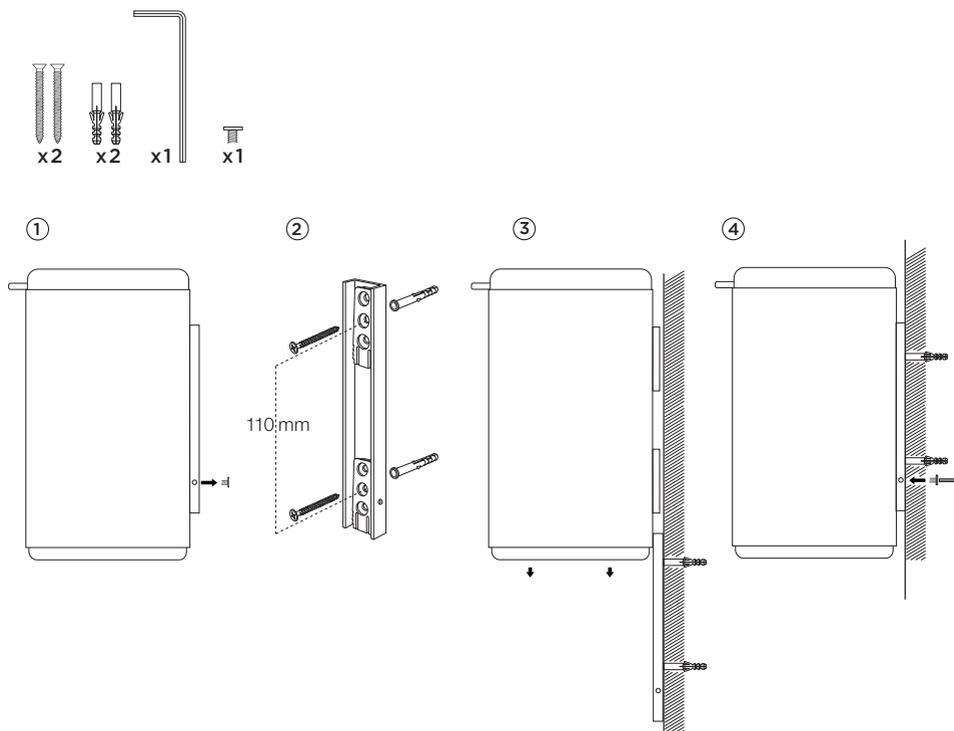
**EN |** Screws and rawplugs for brick walls are included. But please note that there are many different wall materials, so always choose screws and rawplugs that are suited to the relevant wall material and have sufficient bearing capacity.
