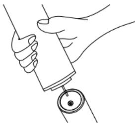
Remove the lid of the refill cartridge and remove any adaptor ring and adaptors present. Adaptors are not usually necessary for refilling the RÖSLE flambé burner. If by chance the nozzle of the refill cartridge does not fit the gas valve of the burner, select the appropriate adaptor ring.
