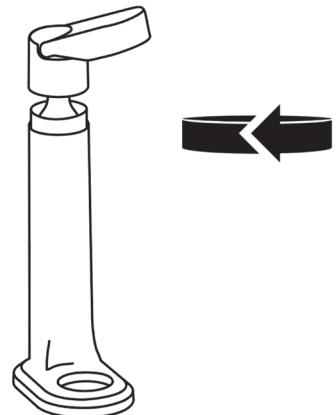
Aim the cylinder connector to the right position with the main body, then turn clockwise to fasten the cylinder connector and the main body.
