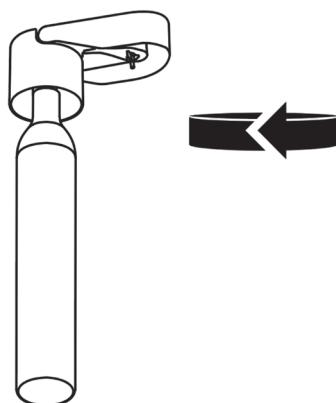
Remove the dust-proof cap from the CO<sup>2</sup> cylinder, unscrew the cylinder connector from the body. Hold the cylinder connector in one hand, and with another hand screw the CO<sup>2</sup> cylinder clockwise into the cylinder connector till fastened.
