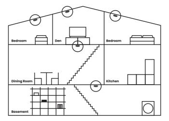
A Smoke Alarm should be placed next to each bedroom and there should not be a distance greater than 10 meters between each Smoke Alarm. Additional security can be achieved by installing Smoke Alarms in all rooms. However, it is not recommended to install Smoke Alarms in kitchens, bathrooms or garages, where steam, smoke and exhaust can trigger the alarm.
