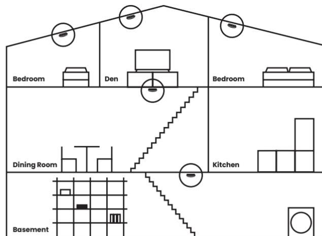
A Smoke Alarm should be placed next to each bedroom and there should not be a distance greater than 10 meters between each Smoke Alarm. Additional security can be achieved by installing Smoke Alarms in all rooms. However, it is not recommended to install Smoke Alarms in kitchens, bathrooms or garages, where steam, smoke and exhaust can trigger the alarm.
