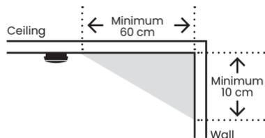
It is not recommended to mount the Smoke Alarm at the top of a pointed ceiling, or in a location in a dead angle, where the smoke will not collect.
