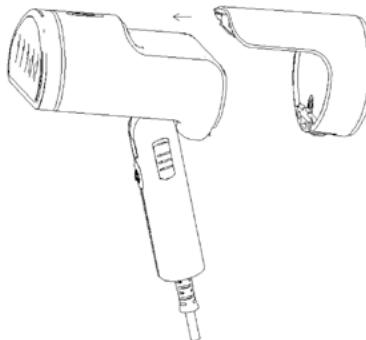
**Drainage:** Hold the tank lock and pull back, open the lid the bottom of the tank, drain the remaining water and install the lid back tightly, then fill the tank.
