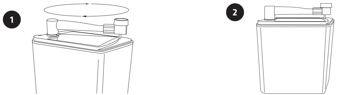
**EN** Turn the cheese slicer clockwise to cut slices from the cheese. The base is automatically drawn upwards each time a slice of cheese is cut.
