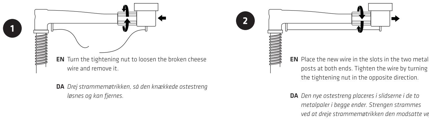
**EN** If the wire or metal post at the end of the cheese slicer arm scrapes against the cheese box, it may be because the wire is too tightly tensioned. This can be remedied by slightly loosening the wire.
