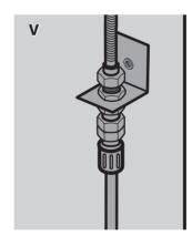
V) Both screw connections on the multiple connector (the connector is on the right-hand side wall of the cabinet)
