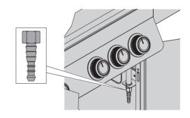
The 30 mbar models come with a universal adapter to connect the gas hose from the pressure regulator to the hose leading to the burner.
