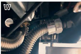
W) Connection between the corrugated hose and the valve unit (the connection is on the right-hand side under the control panel)
